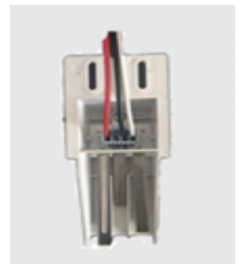
P. Disassembly completed For cleaning the water level sensor separately, Pull the edge of the hook by a screw driver and lift the sensor pin up as shown in the picture The 3 sensor pins are to be cleaned in the same way
